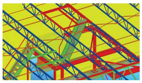
Digital joist design supports early collaboration on BIM-based steel joist design integration. Shown here is a screen capture taken from New Millennium's Dynamic Joist steel joist modeling program, a component plug-in to Tekla Structures.
