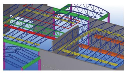
Example showing objects being coordinated through/around joist webbing. New Millennium Building Systems
