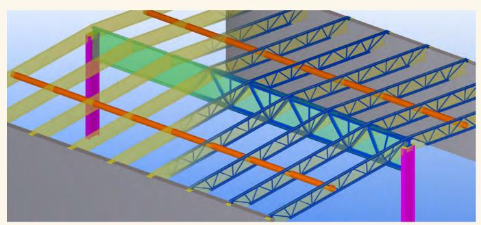
A basic advantage of our digital steel joist design software has been the ability to move from generic representations of a structure, to seeing and verifying all structural elements by way of spatially accurate, three-dimensional objects.
