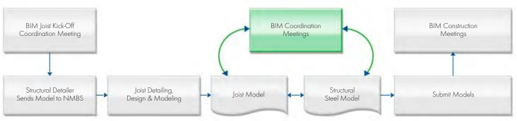
New Millennium's process for steel joist BIM development is a significant improvement over the traditional RFI approach to structural steel project design and delivery, because it brings more clear, model-guided procedures, communication and accountability.
