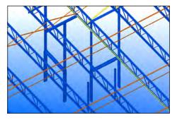
The as-built steel joists design enabled the structural engineer/detailer to design the reinforcement for this door framing, including bolting details.
