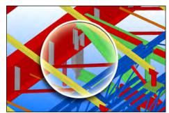
3D model revealed a stabilizer was not planned for this joist girder. The engineer designed a stabilizer hanger for the bottom chord extension, preventing a field erection problem.
