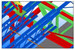
The 3D model enabled the structural detailer to coordinate with the steel joist detailer to extend the bottom chords of these double joists, for added reinforcement.
