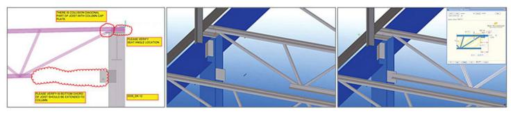
These images depict error detection in the digital realm: A question regarding apparent missing joist information is shown (left), the area was located in the model (middle), and determined that the section information for that joist was incorrect. The problem was quickly and easily corrected and visually confirmed (right).
