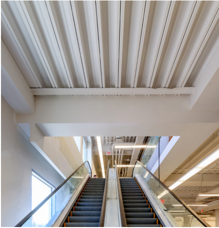
Architectural deck is often left exposed to present a bold ceiling pattern. Deck can be painted by the factory for long-term protection.
